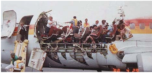
Fig. 15 Damage caused as a result of crevice corrosion in the fuselage of the Aloha Airlines Flight 737 [44]
