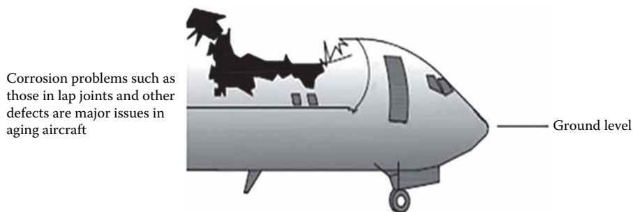
Fig. 14 Schematic description of the Aloha aircraft incident
